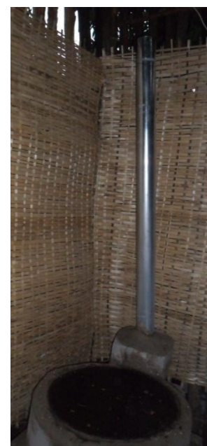
Figure 3.4: injera stove with chimney structure, HH37.
